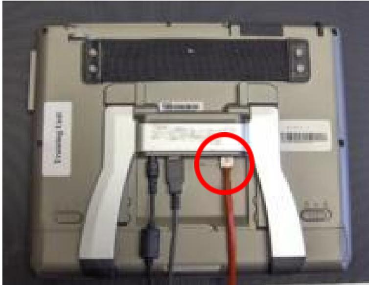
4. Install the protective cover as shown below to help prevent disconnection.
