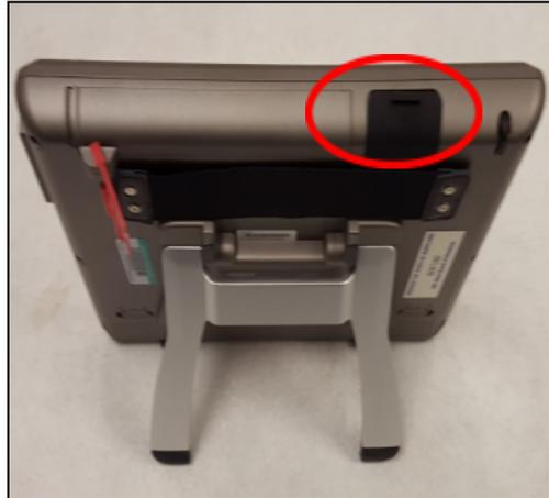
8. Insert the power cord (marked with yellow tape) into the first connection slot marked with PWR. Plug the other end into a power source. **Do NOT turn on the power switch yet!**
