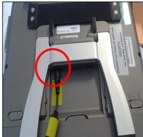
9. Take the printer's USB cable from the printer case. Plug the larger end into one of the two USB ports located on the back of the pollbook. It does not matter which USB port you use.
