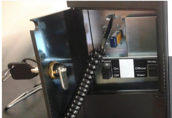
5. Flip the **“Power”** switch to the **“Off”** position.
