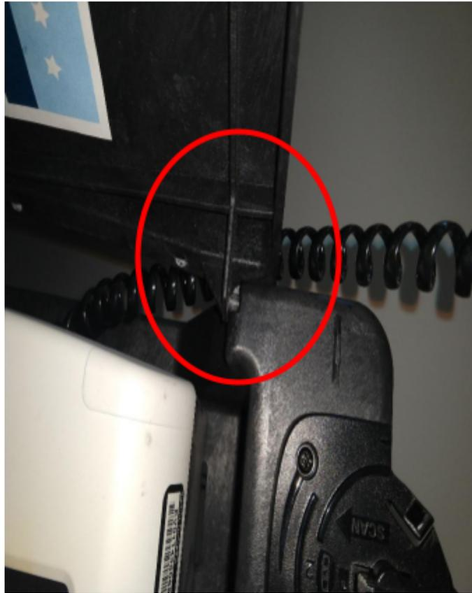
16. Plug the headphones into the audio port located on the front of the ballot marking device.
